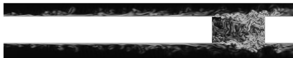
Figure 10. VALIANT ‘gap – turbulence interaction’ case: SA IDDES ( Re = 2 \cdot 10^4 ), vorticity magnitude in the central cross-section. The Cartesian mesh of 8.4 million nodes and 49.5 million tetrahedrons.
